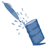
4 drops of ink in one 55-gallon barrel of water (thoroughly mixed) makes an ink concentration of 1 ppm
